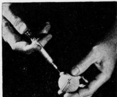
This shows the needling process in its experimental stage. It is now done mechanically.
