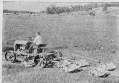
For transporting, the mowers are swung around behind, and the total width is less than that of a three-unit outfit.
