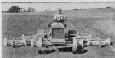
Note the arrangement of the two front mowers, which cut the grass before it is matted down by the drive wheels.
