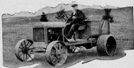
The new Toro Junior Model B-30 has a wheel base of 98 inches, and is equipped with a dump box. Exhaustive field tests have proven that the new Toro will climb a 30% grade with a full body load. Note the trim appearance and well balanced lines.
